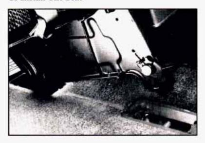
Lower the seat into position. Make sure the front retainers are hooked onto the anchor pins. Pull the seat down to latch the rear retainers. Make sure the seat is locked in by pulling up and down on the seat.
